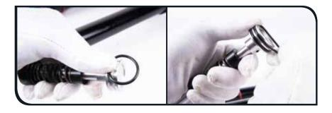
Apply the grease to the air piston and the spring.
