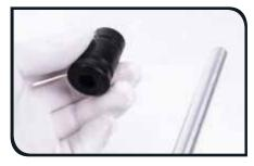
Use the 24mm sleeve to remove the top cover. Apply grease to the top cover o-ring.
