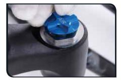
Remove the air valve cap.
