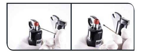
Remove the rebound adjuster knob. Use a 5mm hex wrench to unscrew the bottom bolt.
