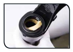
Apply the grease around the wiper seals.
