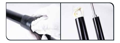
Inspect the tension pin hole on the air piston. If the tension pin is protruding or not centered, replace the air piston. Remove the o-rings from the piston.
