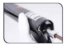
Install the small ball and the small spring. (The damping function is optional.)
