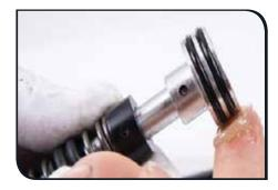
Push the air spring assembly into the bottom of the upper tube.
