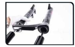
Remove the rubber bumper from the air shaft.
