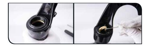
Remove the foam rings. Spray the foam rings with isopropyl alcohol.(The foam ring is optional accessory.)
