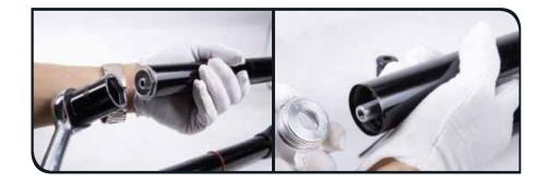
• Use pliers to remove the air spring assembly.
