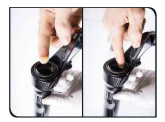
Install the rubber bottom out bumper on the air shaft.
