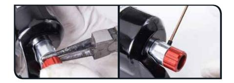
Pump the air with professional air pump. Follow the suggested air pressure chart. Install the air valve cap.
