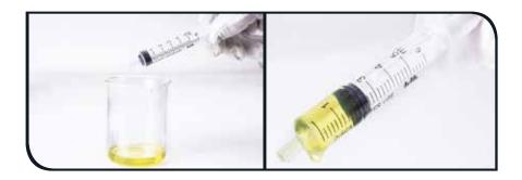
Inject the fork oil to the upper tube, make sure the oil covers the piston.
